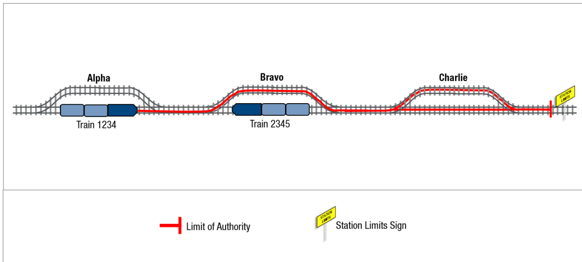
Figure 5017-9 Train No 1234 has an Authority to Proceed to Bravo, take Loop, cross Train No 2345 then Proceed to Charlie. The condition to depart Bravo is that Train No 2345 has arrived complete at Bravo.
