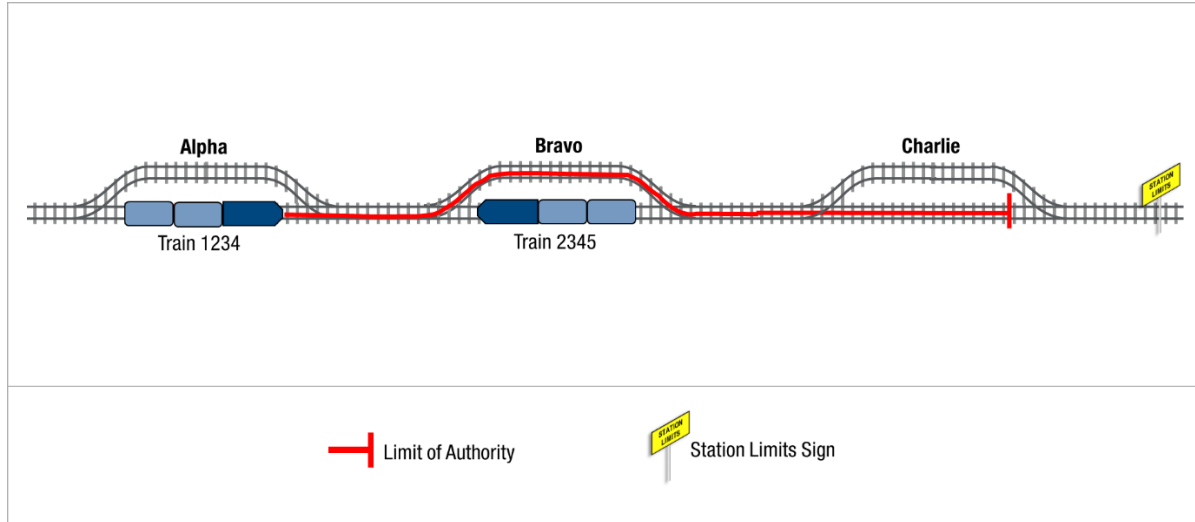
Figure 5017-9 Train No 1234 has an Authority to Proceed to Bravo Loop, Cross Train No 2345 then Proceed to Charlie. The condition to depart Bravo is that Train No 2345 has arrived Complete at Bravo.
