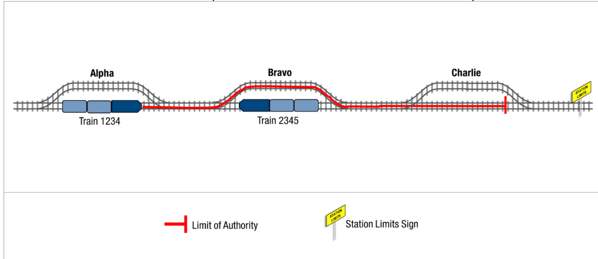
Figure 5017-9 Train No 1234 has an Authority to Proceed to Bravo, take Loop, cross Train No 2345 then Proceed to Charlie. The condition to depart Bravo is that Train No 2345 has arrived complete at Bravo.
