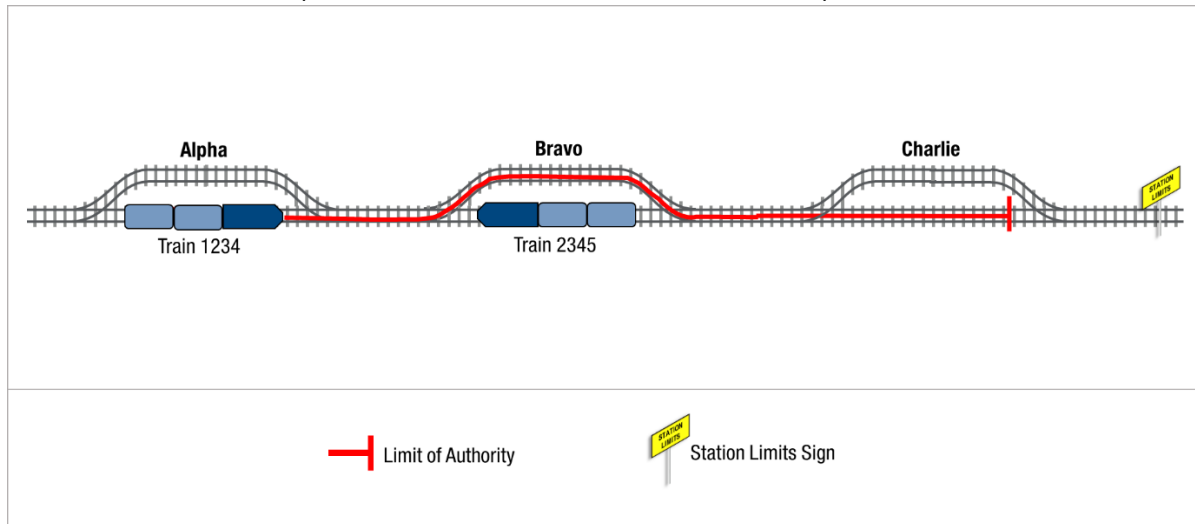
Figure 5017-9 Train No 1234 has an Authority to Proceed to Bravo Loop, Cross Train No 2345 then Proceed to Charlie. The condition to depart Bravo is that Train No 2345 has arrived Complete at Bravo.
