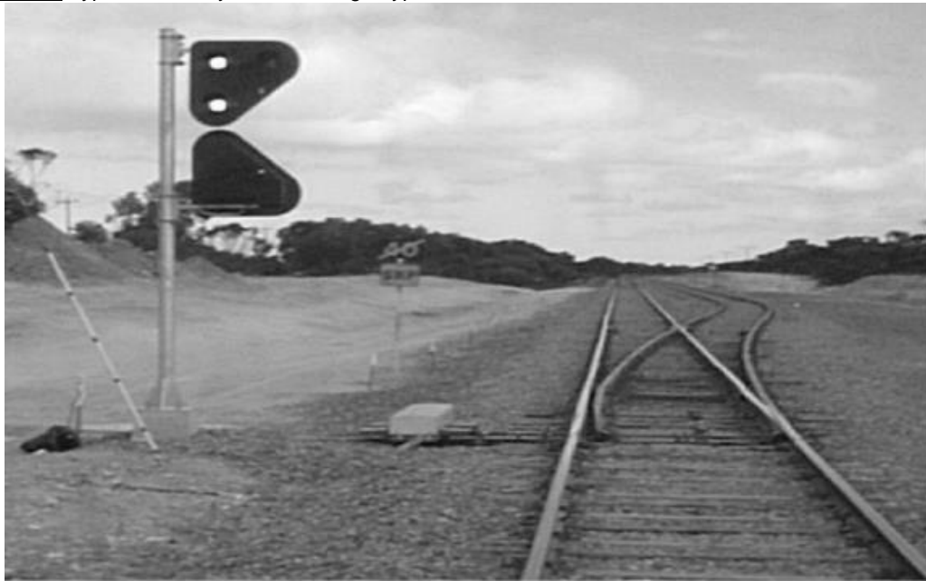
Figure 9022-1 Typical SRP Layout – white light type
