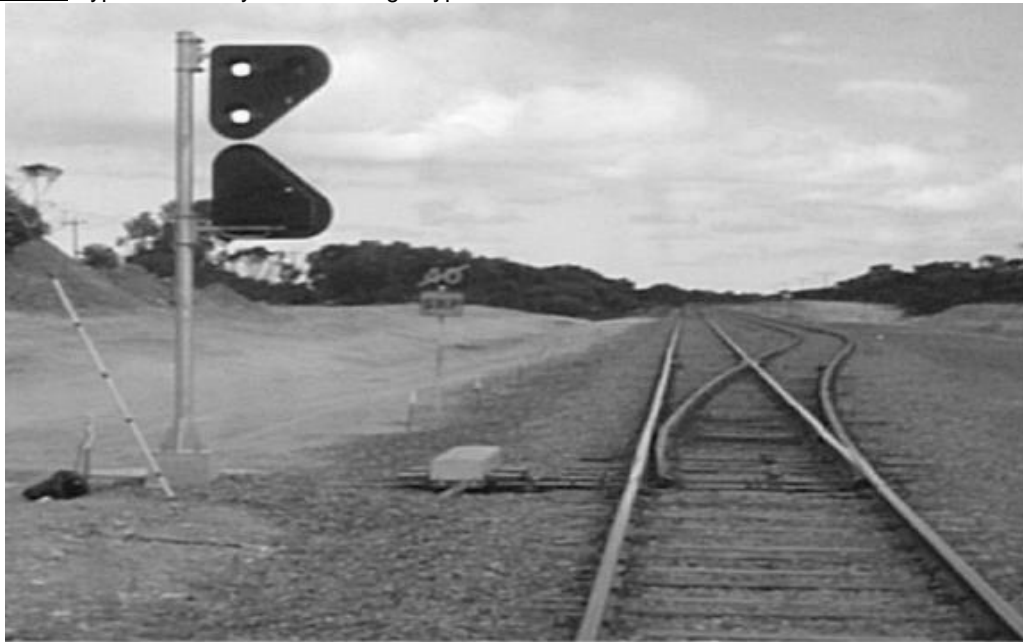
Figure 9022-1 Typical SRP Layout – white light type
